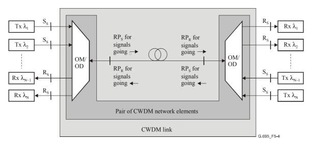
Figure 5-4/G.695 – "Black Link" approach for bidirectional applications
