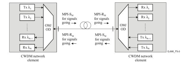
Figure 5-3/G.695 – "Black Box" approach for bidirectional applications
