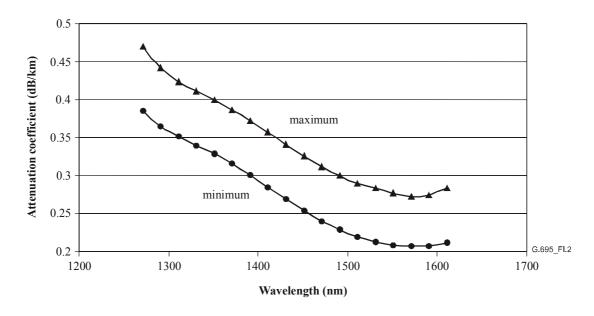
Figure I.2/G.695 – Assumed attenuation coefficient values for G.652.C and D cable
